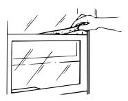
Slide the air conditioner into the case and replace the front grille. Install the two ground/anti-theft screws removed at the beginning of the installation.
